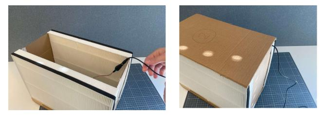
7) Tape the bottom of the purifier, starting with the wire, using the same method as in step 5).
