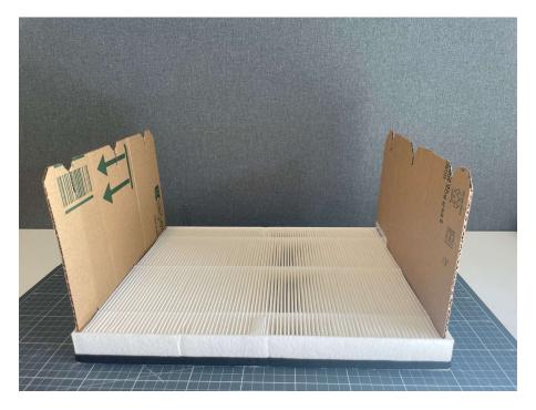
Don't hesitate to trim corners a little more or widen slots if inserting parts (3) is difficult. Be careful not to bend the cardboard.
