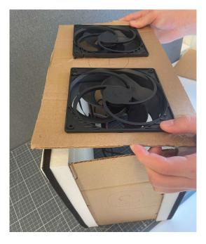
5) Tape the top of the purifier all the way round, leaving half the tape sticking out, as shown in the photos.
