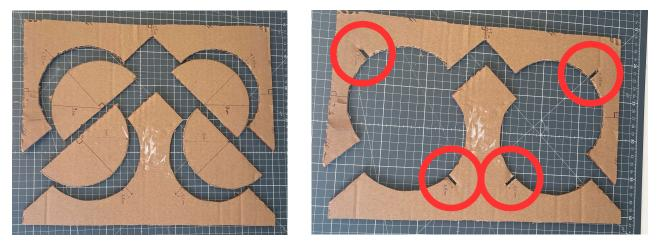
Technique for making the slits: make small cuts 1mm to the left and 1mm to the right of the line, then tear the tab by hand.
